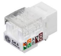
When terminating the IDC terminal connections it is important to use the correct insertion tool. Excel recommend either a standard 110 insertion tool and blade (or BK insertion blade). The wires must be trimmed closely to the jack body using sharp flush cutters.
